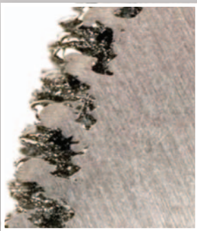
Continuous Trabecular Titanium trabecular structure
