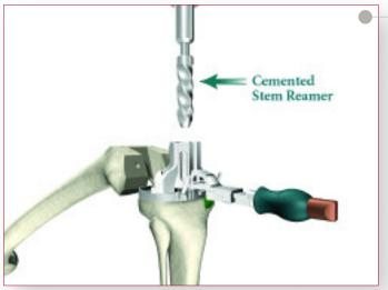
▶ Attach the appropriate Cemented Stem Reamer to the Universal Driver. Place the Cemented Stem Reamer into the Keel Punch Guide, inserting the Cemented Stem Reamer Bushing into the central hole of the Keel Punch Guide.
